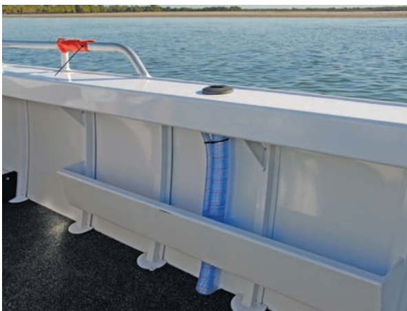
A two metre long side pocket is installed to port within the main cockpit area.
