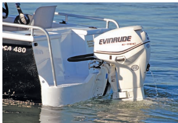
Left: While minimal power the 60 E-Tec had no problems in powering the craft at speeds up to 50km plus.
